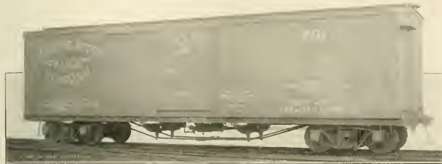
BOX CAR WITH STEEL FRAME, 100,000 POUNDS CAPACITY.
